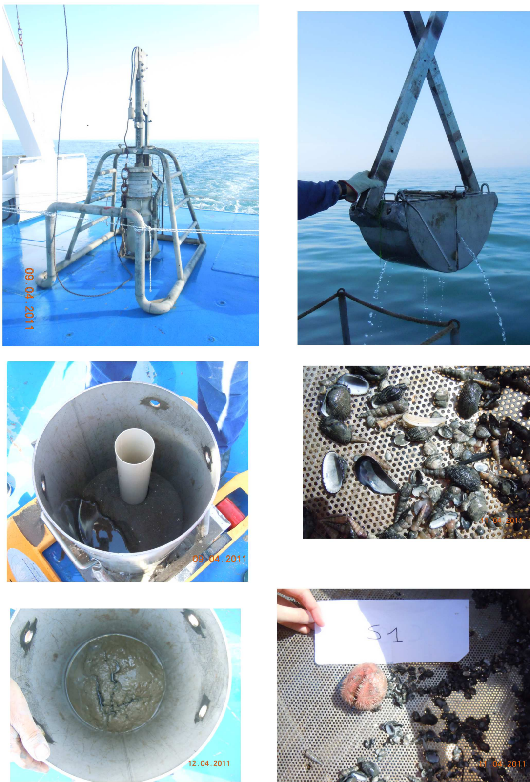
Figure 14. Cruise ENVADRI2011: Bottom sampling by Oceanic Box-Corer and grab.
