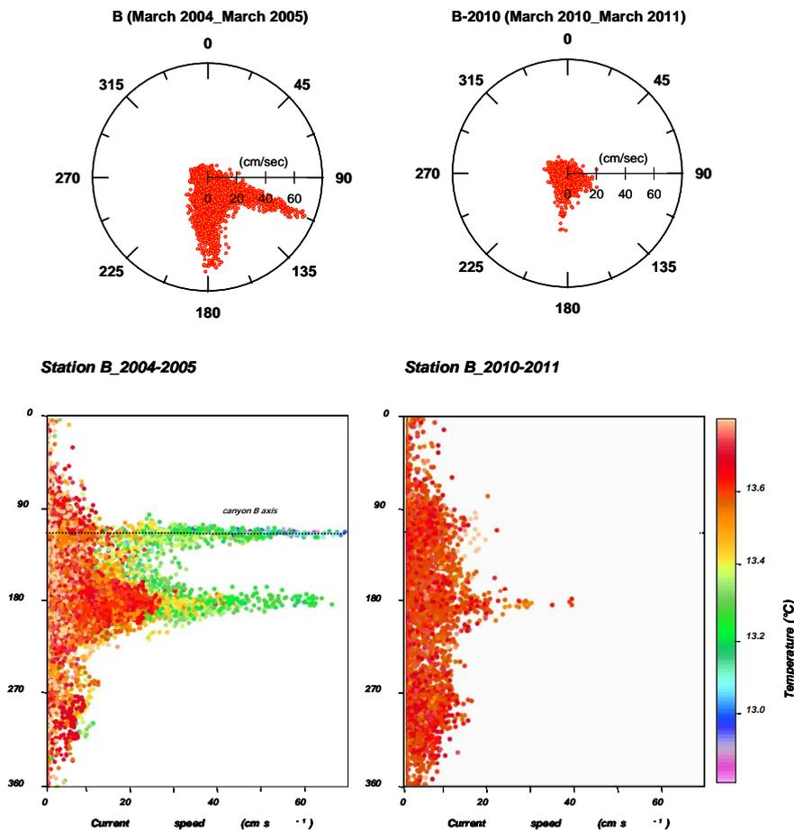
**Figure 5.3** Currents (speed and directions) and water temperatures measured at site B during 2004-2005 and 2010-2011.
