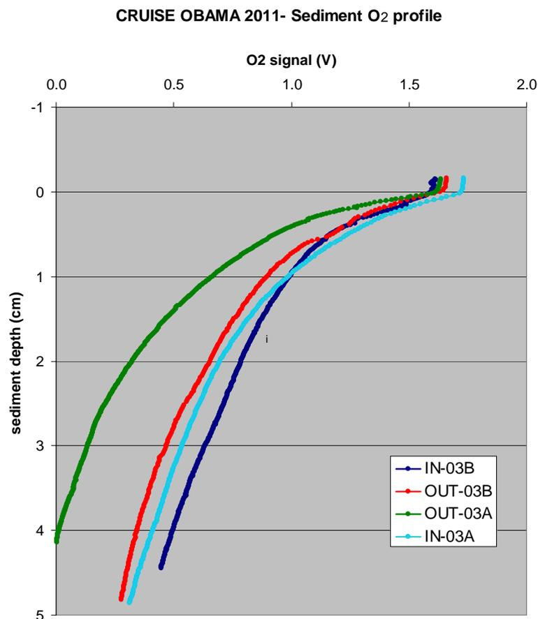
**Figure 6.3.** Oxygen microprofiles measured shipboard on SML area
