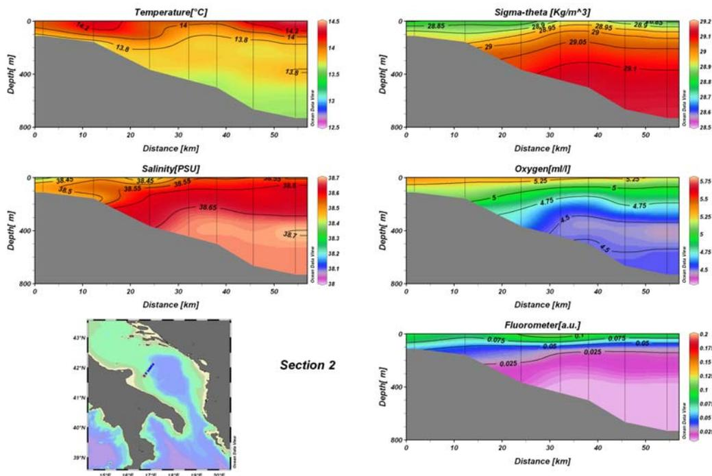
**Figure 3.3.** Temperature, salinity, sigma-theta, dissolved oxygen and fluorescence distributions at section 2.
