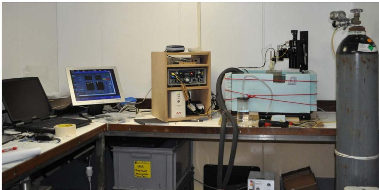
**Figure. 6.2.** Set-up of the experimental system for measuring oxygen microprofiles in a sediment core. The sediment core is positioned within a thermostatic water bath kept at the temperature of the sea bottom.
