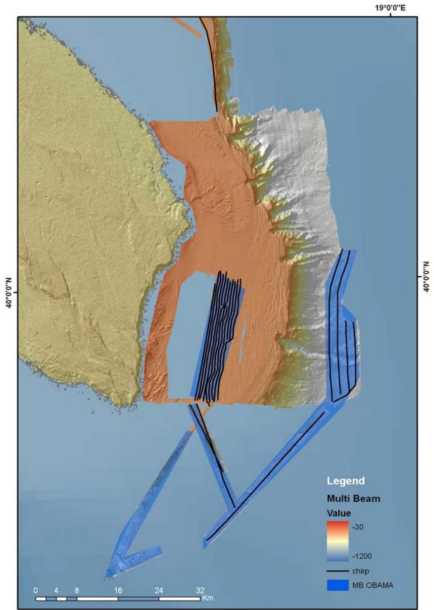
**Figure 2-1.** Chart of Chirp profiles and Multi beam coverage
