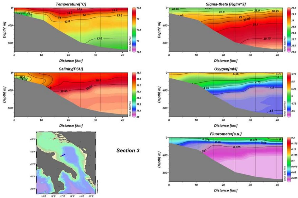
**Figure 3.4.** Temperature, salinity, sigma-theta, dissolved oxygen and fluorescence distributions at section 3.
