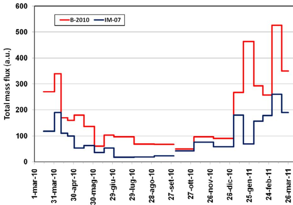
**Figure 5.5.** Total mass fluxes, measured in arbitrary unit, at sites B and IM7 in 2010.
