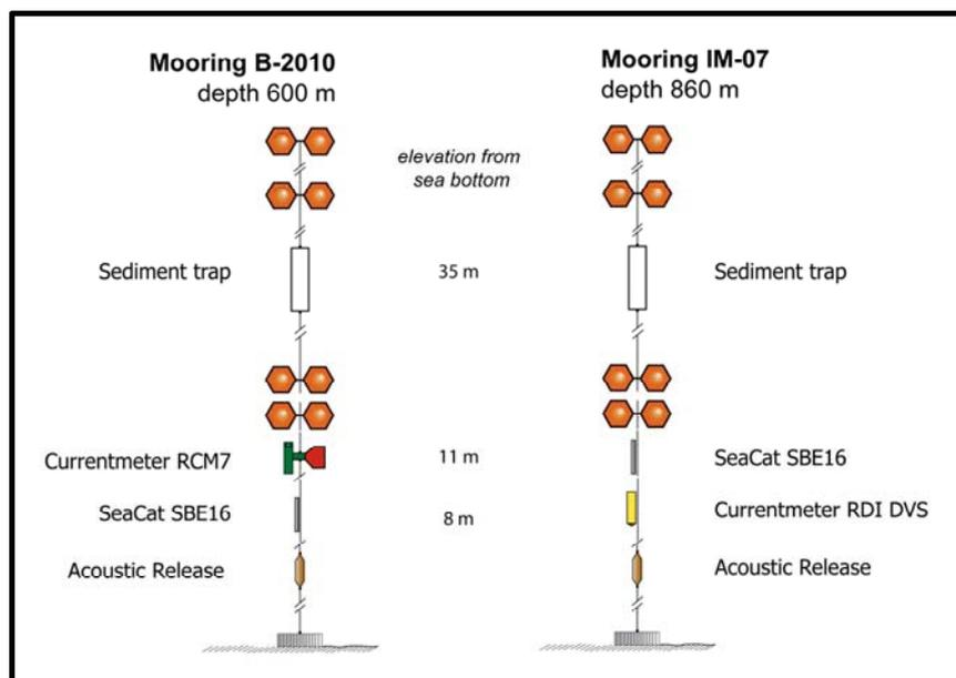
**Figure 5.2.** Configuration of the recovered moorings. B-2010 mooring is working in the southern branch of the Bari canyon, while the IM7 mooring was deployed in the sediment waved field down current to the Bari canyon.
