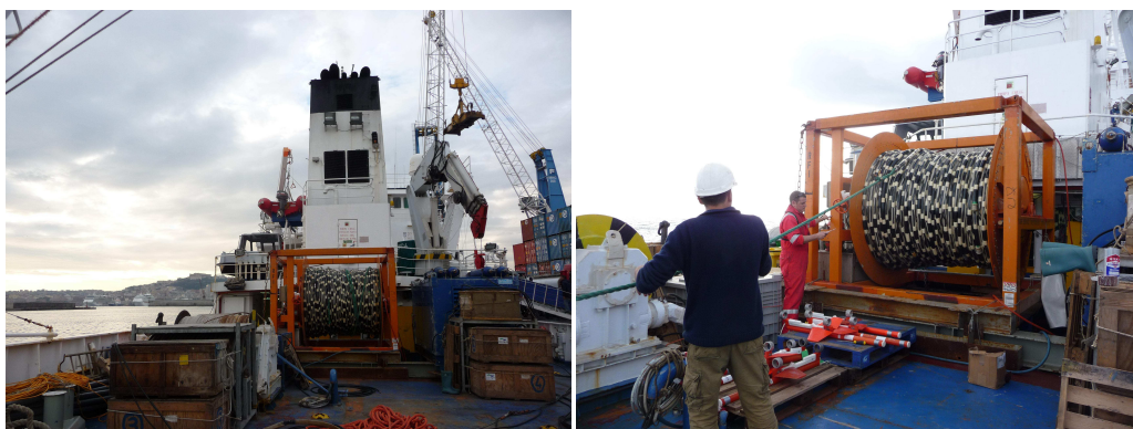
Figure 6: The EEL streamer (Sercel 96 channels digital) and DIGICOURSE Cable Levelers.
