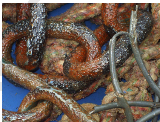
Figure 26. Recovery buoy E1, rusted chain, ~ 3 m below buoy, R/V Mariagrazia , LTES1-10.
