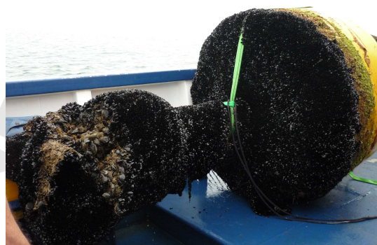
Figure 14. Buoy E1, recovered, on bridge. Note the cover of mussels and other biological material, R/V Mariagrazia , LTES1-10.
