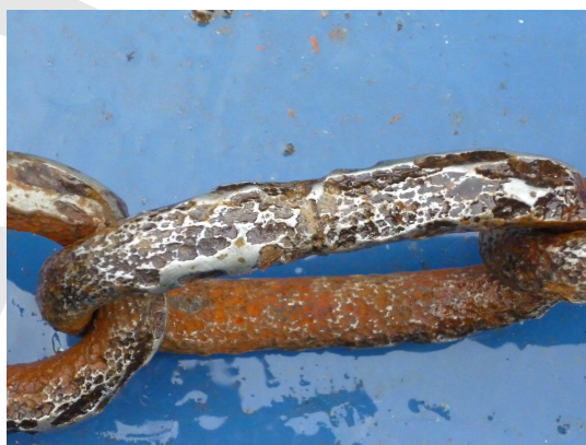
Figure 27. Recovery buoy E1, rusted chain, ~ 3 m below buoy, R/V Mariagrazia , LTES1-10.
