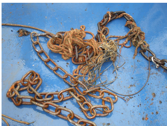
Figure 24. Recovery buoy E1, rusted chain, ~ 3 m below buoy, R/V Mariagrazia , LTES1-10.
