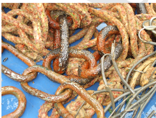
Figure 25. Recovery buoy E1, rusted chain, ~ 3 m below buoy, R/V Mariagrazia , LTES1-10.
