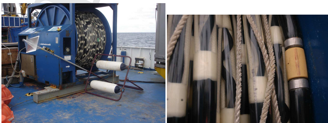
Figure 7: The EEL streamer (Sercel 96 channels digital).
