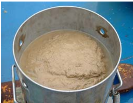
Box core and recovery of undisturbed top to analyse fauna and sediment.
