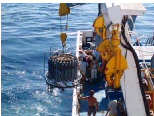
Conductivity temperature depth CTD.
