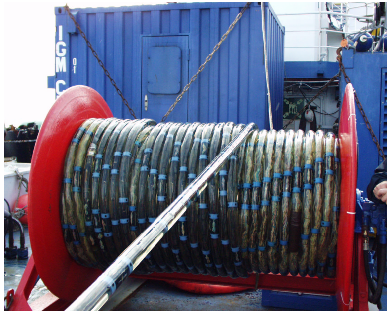
Figure 11: picture of the Teledyne streamer during deployment at sea, taken by S. Carluccio.
