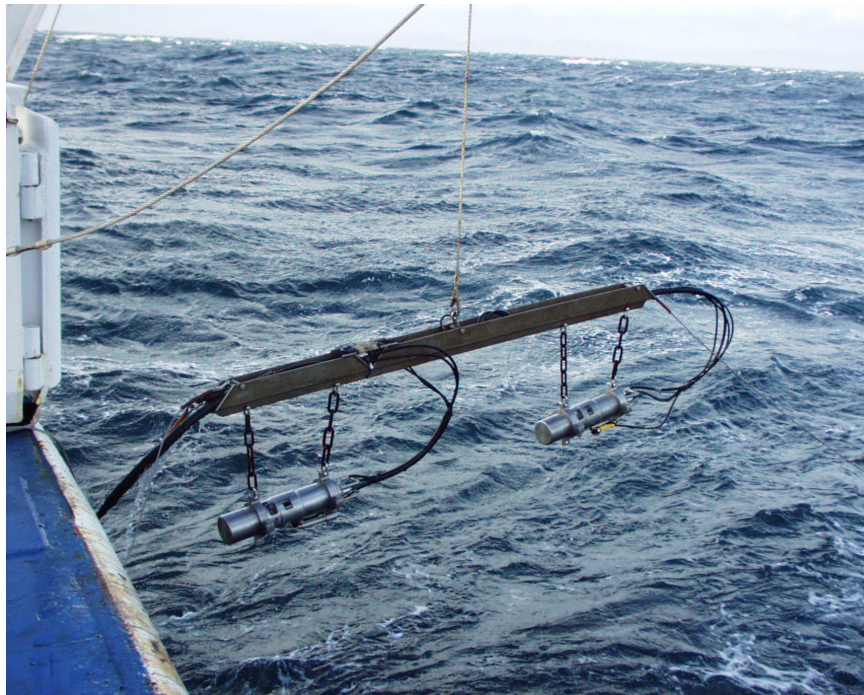
Figure 10: picture of the GI guns during their deployment at sea, taken by S. Carluccio.
