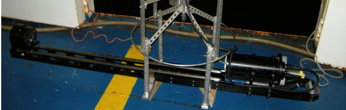
NERONE before deployment GEMS mounted in mooring cage, with its power supply
