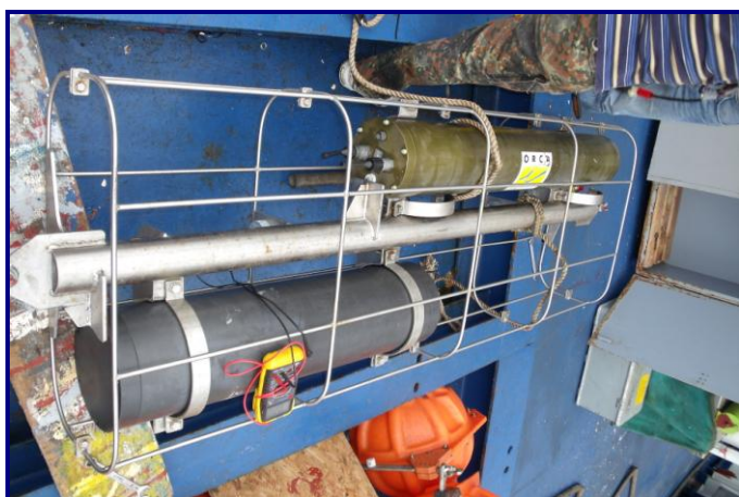
GEMS mounted in mooring cage, with its power supply
