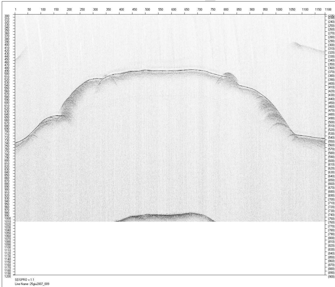
Figure 7: Example of CHIRP SBP acquisition. Unprocessed data, SEG-Y-format.
