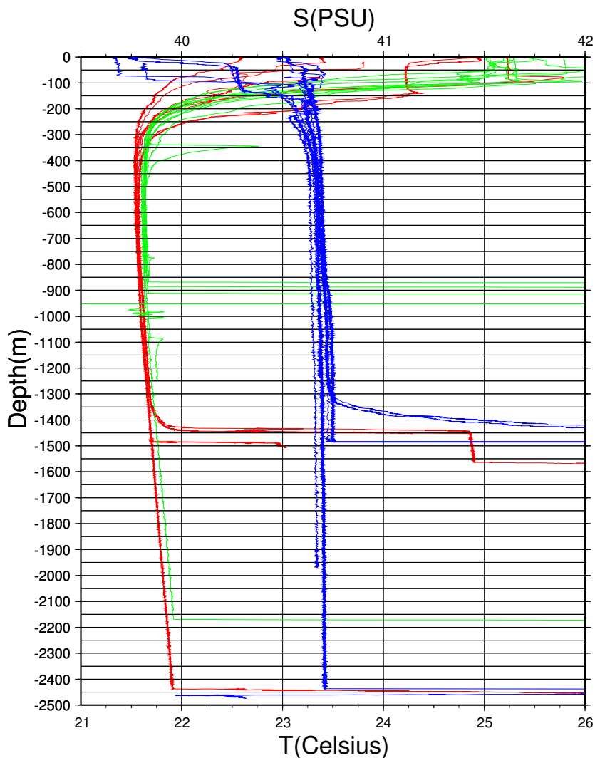
Figure 21: Temperature and Salinity plot of CTD (red, blue) and XBT (green) casts.
