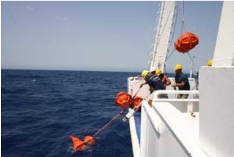
Deployment of the benthic trap buoys.
