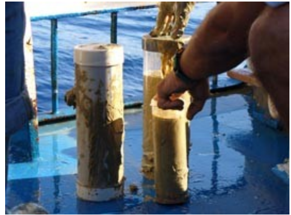
Sediment subsamples from a box core.
