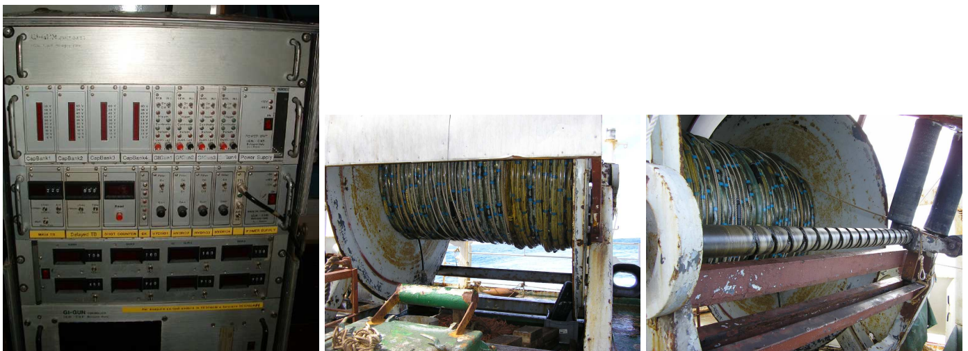
Figure 19: Left: GI-GUN Array Synchronizer. Center, right: Multichannel streamer on Strakhov's winch.
