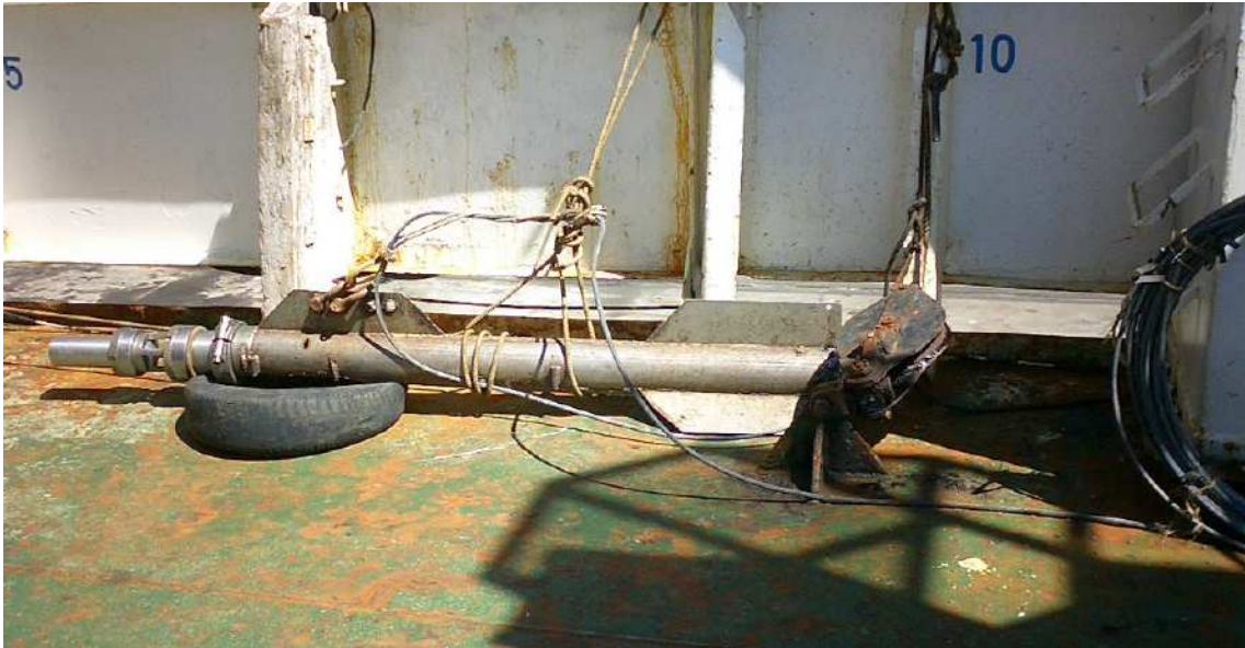
Figure 12: PSK-75 Air-gun (1000ml volume chamber) assembled with tow-system on deck.
