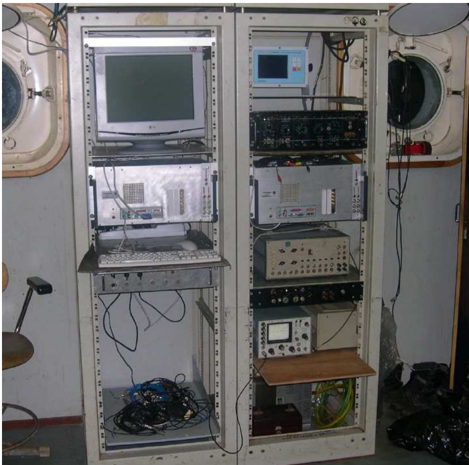
Figure 14: BUP-N instrumental racks. Left (from top): monitor, digitizer SNSP2001/MC1, analog control. Right (from bottom): oscilloscope, solenoid control BUP-4, solenoid control BUP-5, second digitizer SNSP2001/MC-2.
