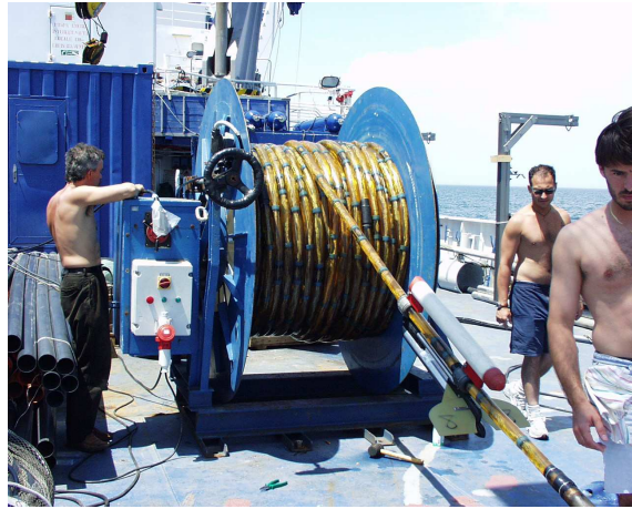
Figure 18: The 24 Channel TELEDYNE streamer. See also the SYNTRON RCL-2 cable leveler.
