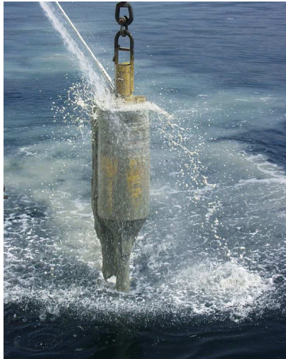
Figure 23: The IGM's 1.2Tons. Gravity Corer.
