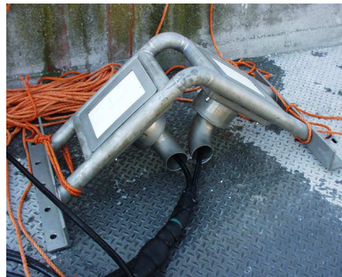
Figure 10: The ELAC/SEABEAM 1180 Transducers mounted on the frame (built by TAINOX) after recovery in Ravenna
