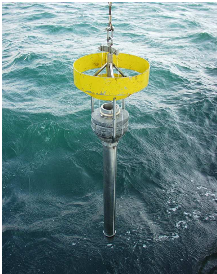
Figure 27: The IGM's Sediment/water SW104 corer.
