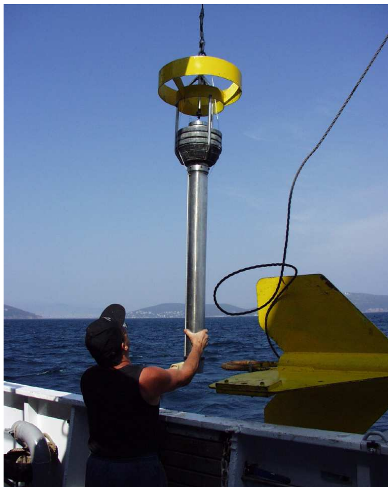
Figure 26: The IGM's Sediment/water SW104 corer.
