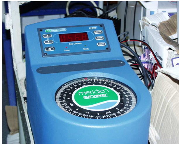
Figure 12: The Meridian Surveyor SG-BROWN with ship docked in Ravenna end of the Cruise. The topographically calculated heading was 58 degrees.
