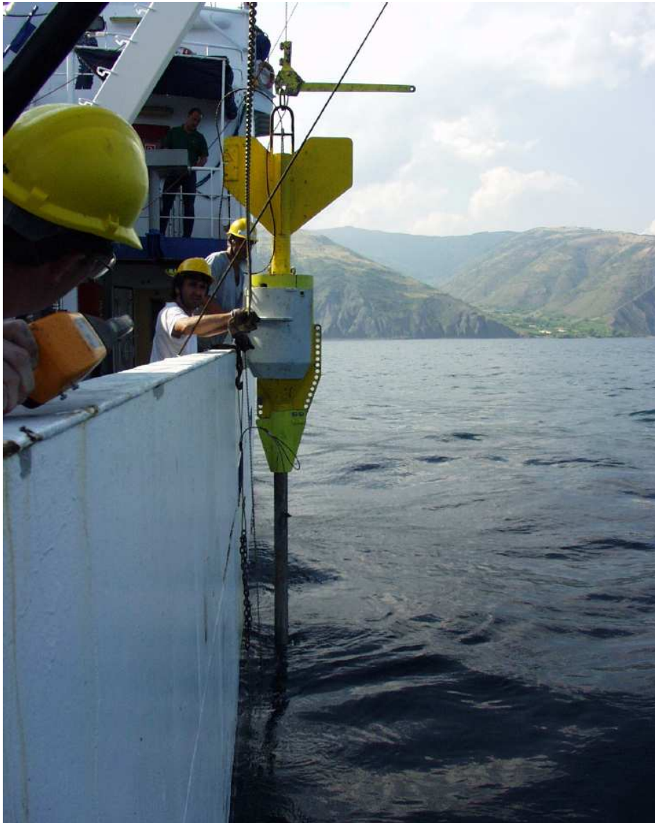
Figure 24: The IGM's Piston Gravity Corer with Free-Fall Trigger.
