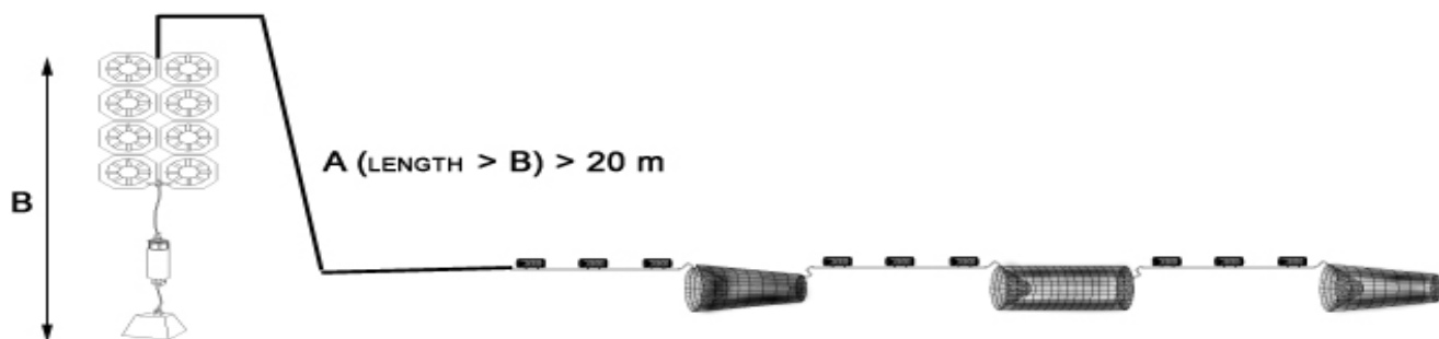
Fig 4. - Temporary Deep Sea mooring scheme.
